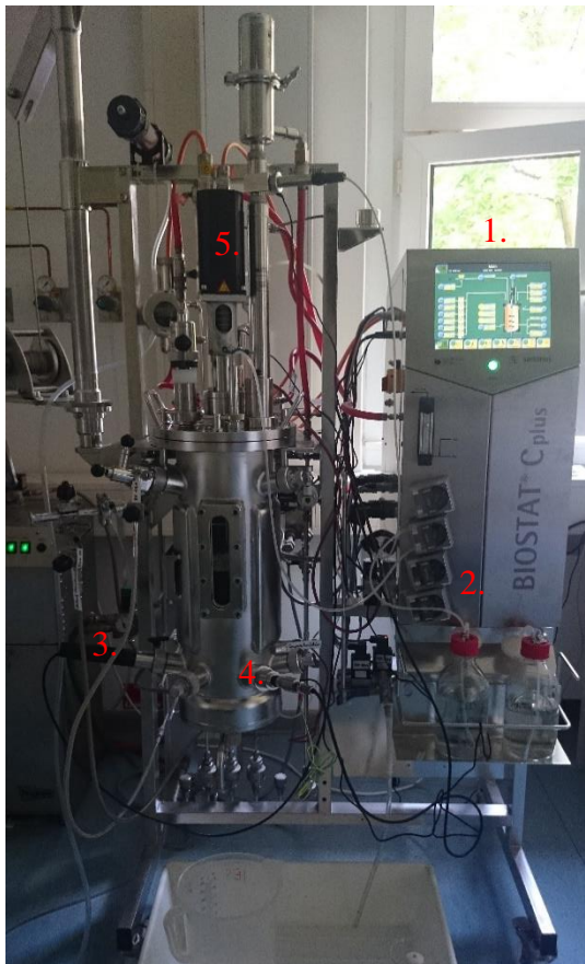
PICTURE 3. Bioreactor set-up used during all the test phases. (1. operating screen, 2. pH regulation, 3. pH sensor, 4. oxygen sensor, 5. stirring)
