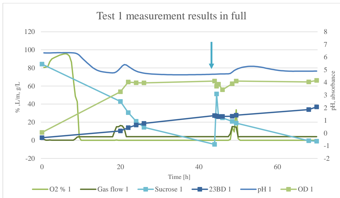
FIGURE 10. The full results of the measurement during test 1. The markers represent the sample collection while the arrow represents the point of feeding.
