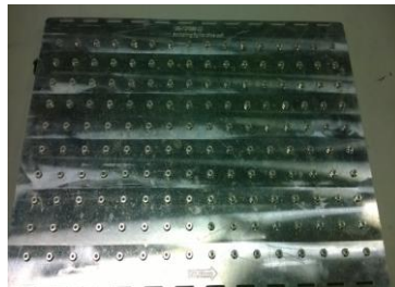
FIGURE 15 b. Automatically put soldering paste
