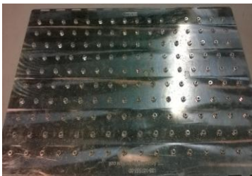
FIGURE 15 a. Soldering paste put by hands paste
