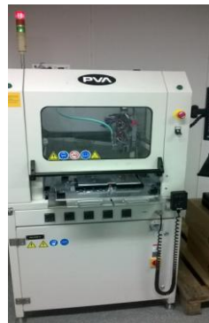
FIGURE 16 b. The new automatic dispenser
