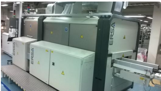
FIGURE 17. The selective wave soldering machine
