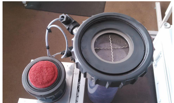
Figure 6. Filter and bottom of the measuring vessel
