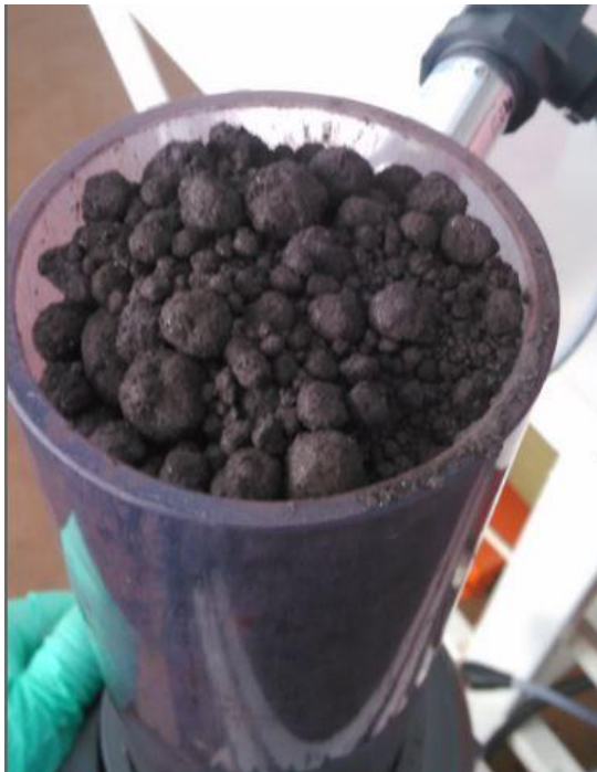
Figure 14. Granulated iron in the measuring vessel of the permeability test rig
