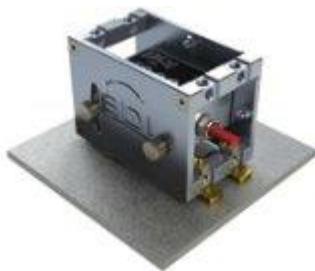
FIGURE 10. Electrolytic tiltmeter by BDI. [29]
