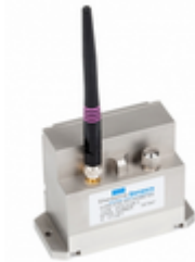
FIGURE 11. Wireless MEMS inclinometer by Sherborne. [31]
