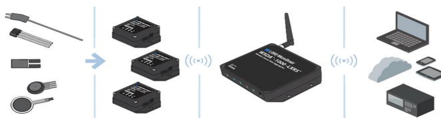
FIGURE 3. Wireless sensor device modularity presented by LORD MicroStrain [9].
