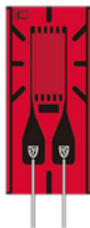
FIGURE 4. General purpose foil strain gauge by Kyowa [12].
