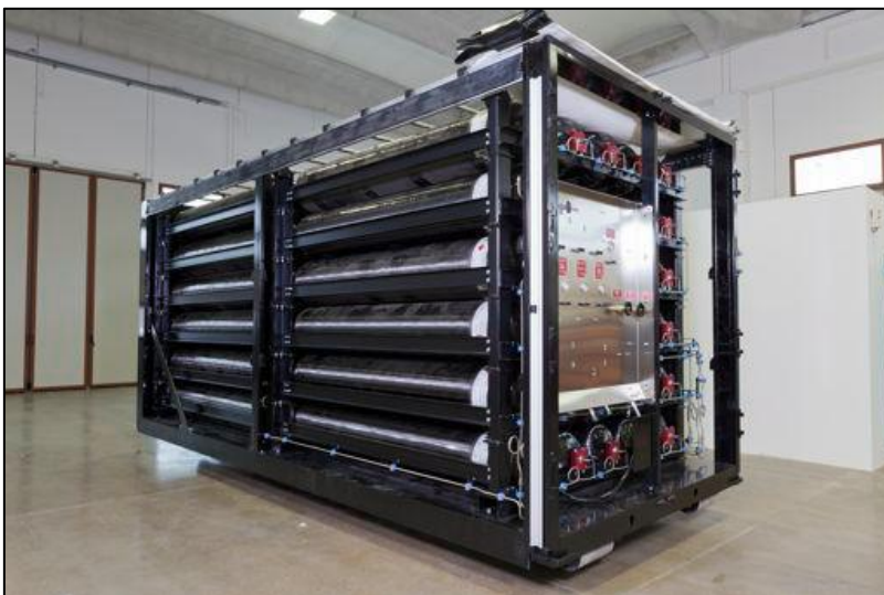
Figur 5. 5045 normalkubikmeter biometan (250 bar) per container.
