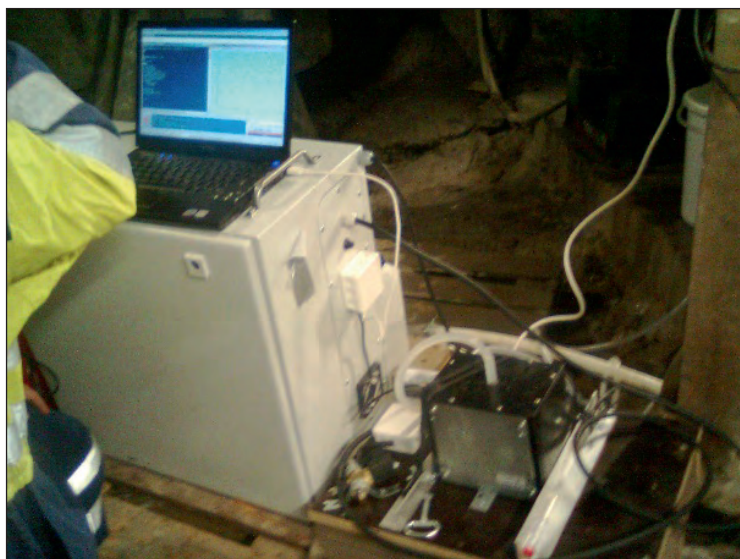
FIGURE 1. The NMR device modified for online measurements in industrial premises (picture Yrjö Hiltunen)
