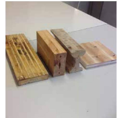
Figure 2. 3D Hot Forming samples (terrace floor, technical beam, I-beam and CLT board) (photo Ilkka Tarvainen)
