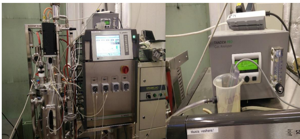
Figure 13: Sartorius Biostat Fermenter with sensor 1 in decanter
