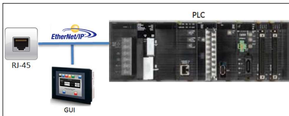
PICTURE 6. Simplified structure of used control system.
