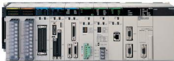
Picture 3. Omron CS1G/H Rack PLC (Omron 2015)
