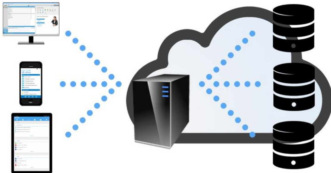
FIGURE 8. M-Files clients (left side) are used to access M-Files Server (center), which manages the document vaults (right side) (M-Files, 2015)
