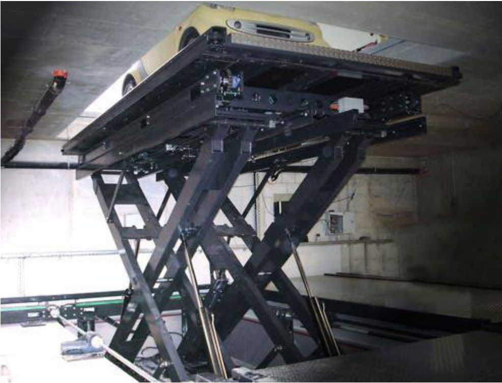
Figure 28 real car elevator
