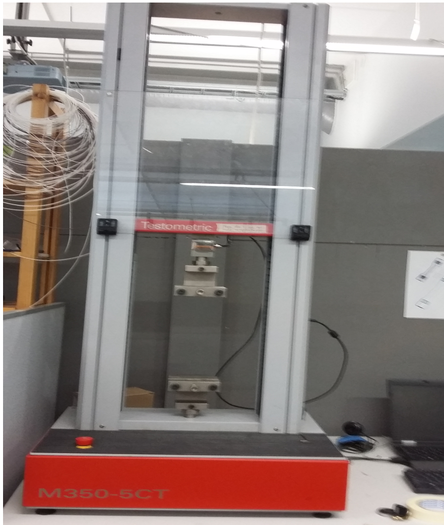
Figure 12: Testometric material testing machine [24]
