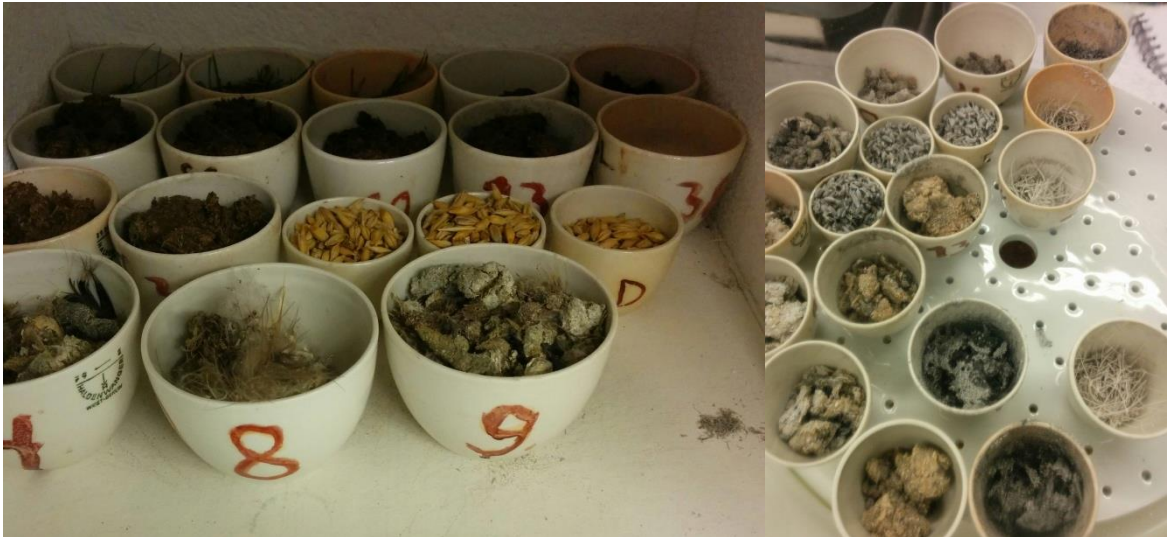
Figure 6: Chicken manure, grain, fox manure 1 & 2, meat and grass in the burning oven (before burning) on the left and in the desiccator on the right.
