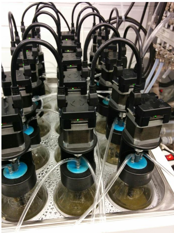
Figure 9: Bioreactors with stirring motors in thermostatic water bath.
