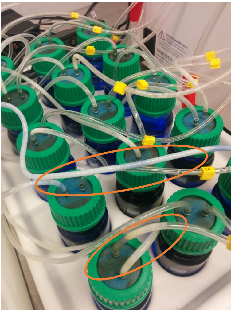
Figure 11: Accumulation of struvite, ammonium carbonate or some other material plugging the pipes (circled orange).
