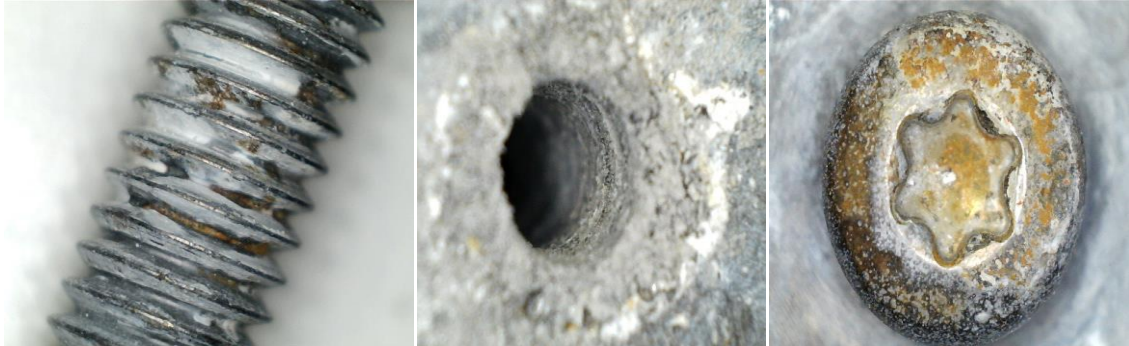
FIGURE 10. 10B21 Zn, thread and head of the screw after salt fog test
