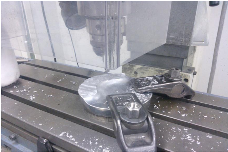
FIGURE 2. Machining of the aluminum plate
