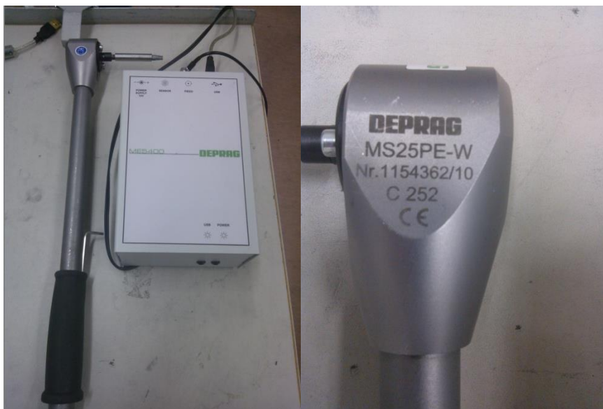
FIGURE 5. Deprag ME5400 measuring equipment
