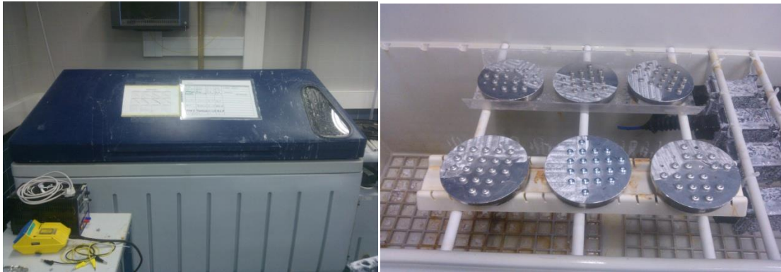
FIGURE 4. Test chamber for salt spray test
