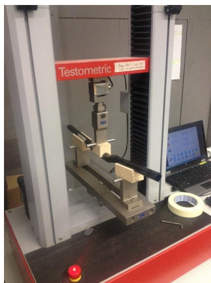
Figure 37: 3-point bending tests setup.
