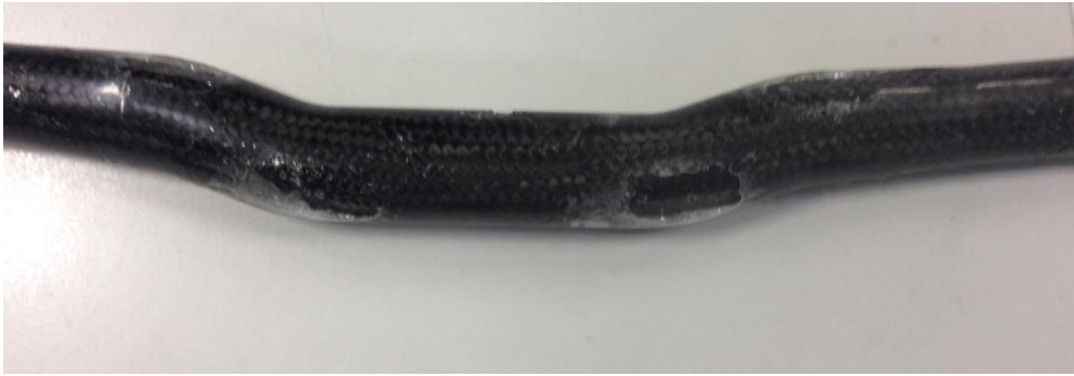
Figure 32: Lamination faults in full sized handlebar, test number 4.
