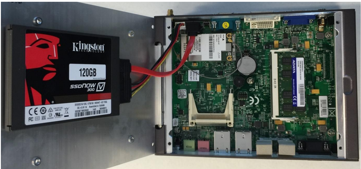
FIGURE 30. Computer unit: Measurements: 20cm x 14.5 cm x 4.5 cm when closed. Features SSD storage and internal SIM card for 3G mobile connection.
