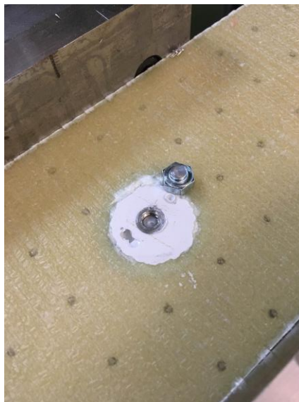
Figure 4-6 Torque test failure
