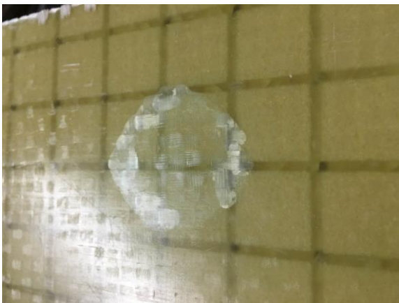
Figure 4-2 Delamination on the bottom
