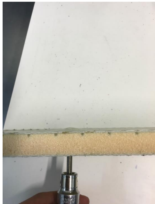
Figure 4-3 Torque test failure
