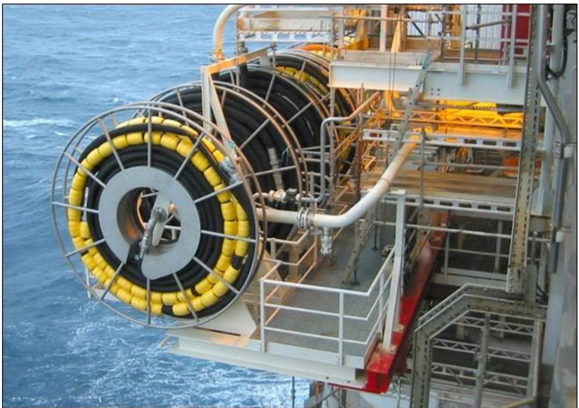
Figure 1. Hose loading station in its working environment (NOV picture archives)
