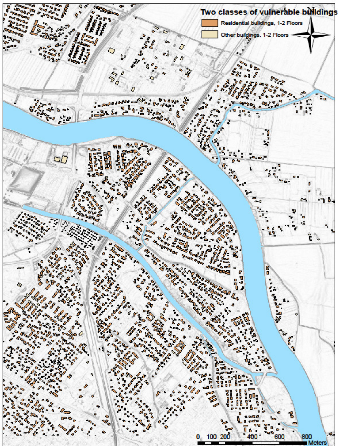
Figure 10: Two classes of vulnerable buildings (Data source SYKE, 2014)
