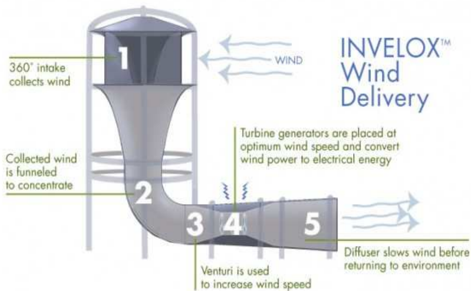
FIGURE 13 Invelox wind delivery system. (Sheerwind, links Technology → How it works.)
