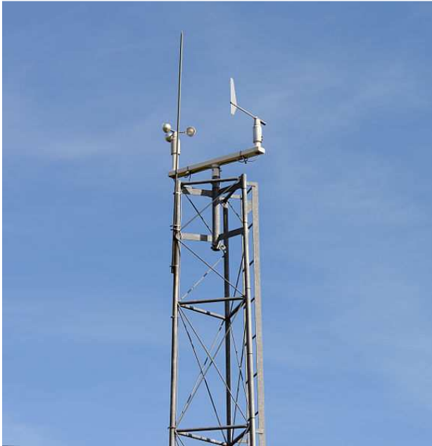
FIGURE 9 Anemometer at the top of the meteorological tower (Luxembourg Beidweiler anemometer.)
