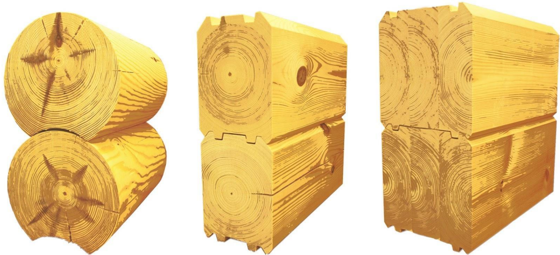
Figure 7. Differences between building log types. From left to right: round log, squared timber, and lamella log. In this case the lamella log has been assembled from three planks, creating two vertical glue layers.
