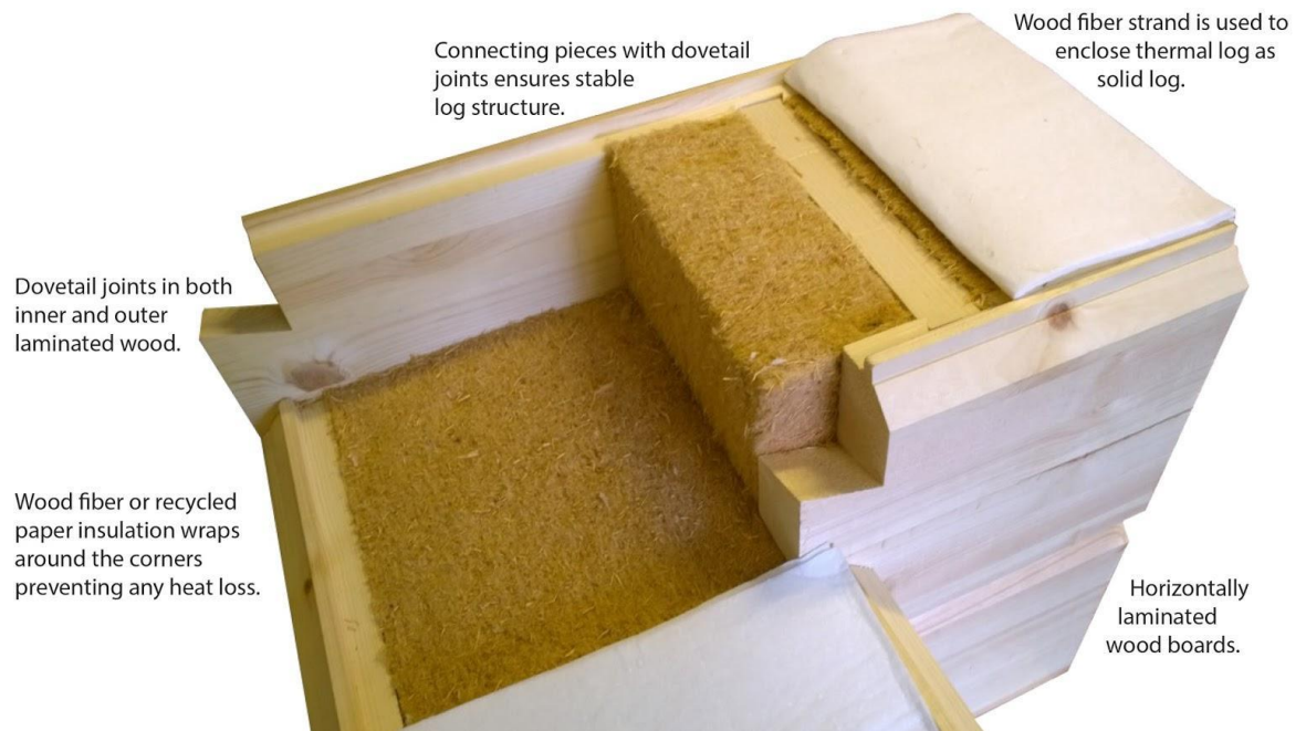
Figure 9. Kero thermal log structure, represented in the corner.
