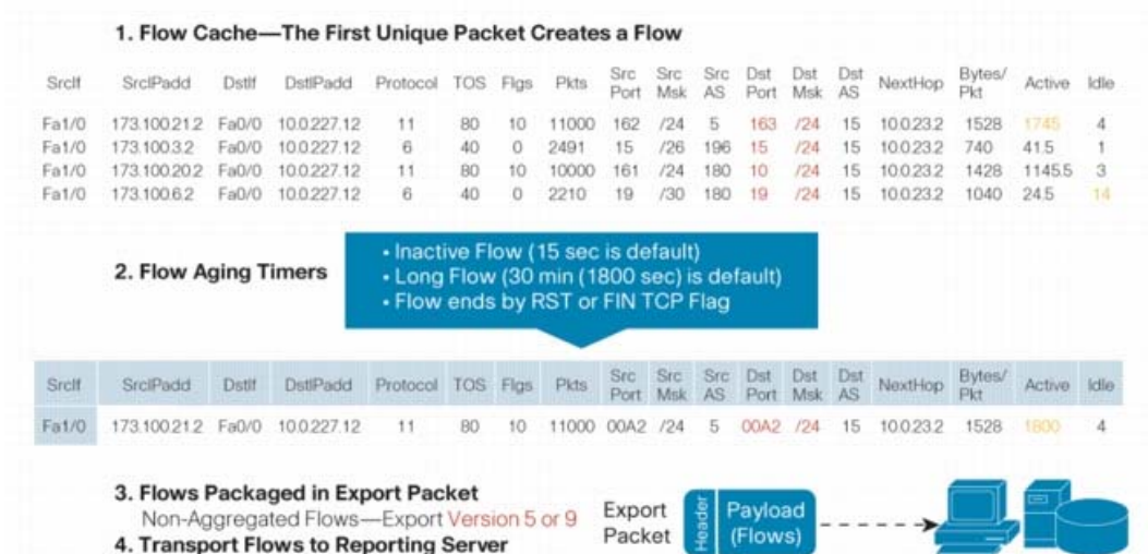
KUVIO 4. Flow Cache (Introduction to Cisco IOS NetFlow - A Technical Overview)
