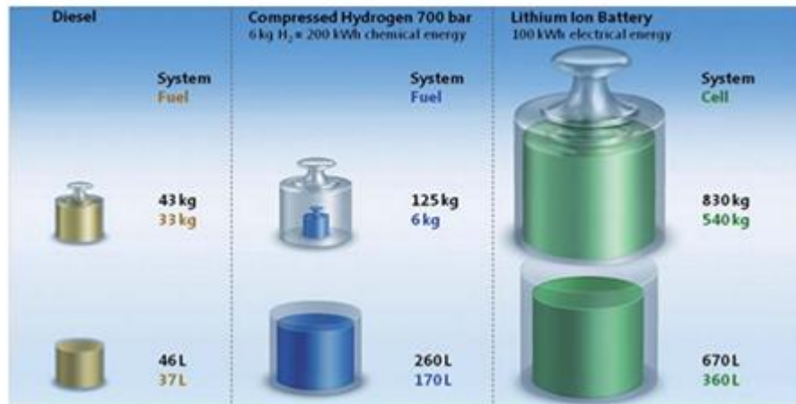
Figure 5. Energy storage system weight and volumes for various energy carriers. [19]
