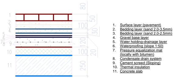
Figure 29. Walkways roof section
