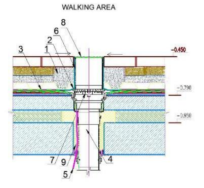
Figure 38. Drainage funnels after repairing
