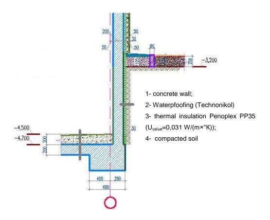
Figure 23. External wall section (parapet wall)
