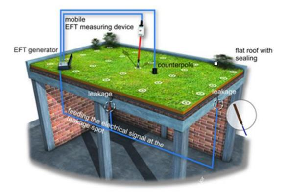
Figure 33. EFT measurements on a flat roof (www.texplor.eu)
