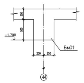
Figure 21. The section of parking roof slab
