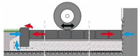
Figure 15. Steering, breaking and accelerating (www.zinco-greenroof.com)
