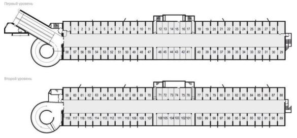
Figure 8. Multistorey parking of corridor type
