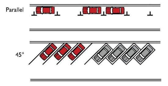
Figure 3. Single level parking of corridor type
