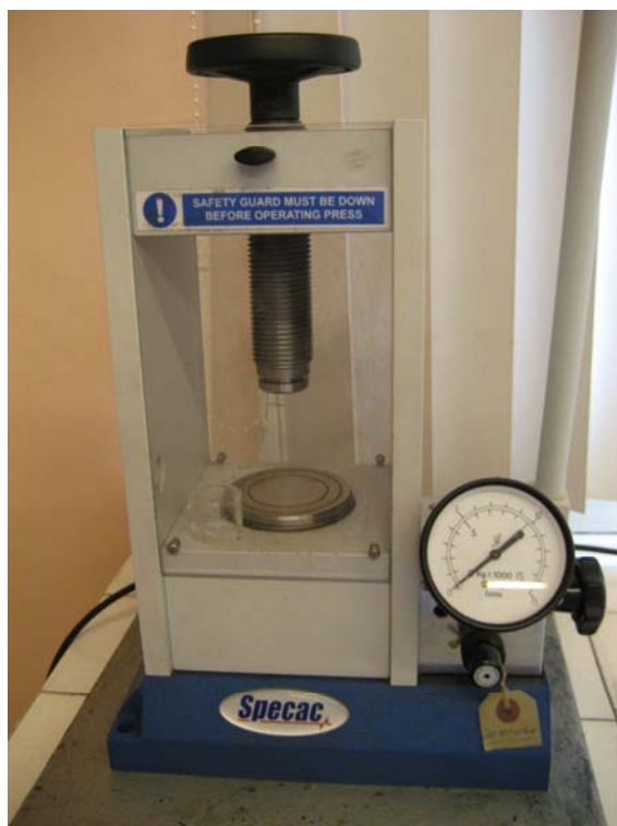
FIGURE 3. Device to prepare tablets for infrared spectra analyses.
