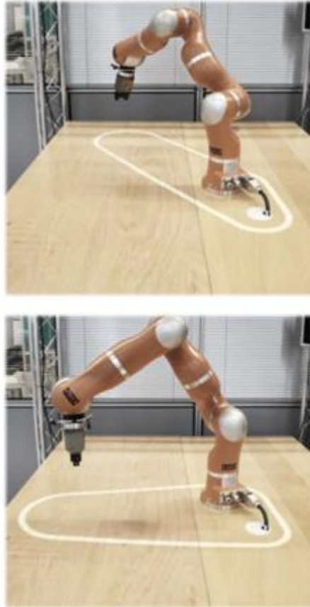
Figure 15 Example of Speed and separation monitoring by Fraunhofer (Fraunhofer 2014a.)
