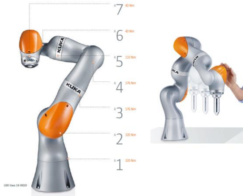
Figure 16 Collaborative robot based on Power and force limiting method by KUKA. (KUKA)
