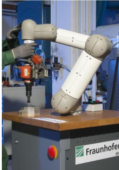
Figure 11: Tactile skin application by Fraunhofer (Fraunhofer 2014b.)
