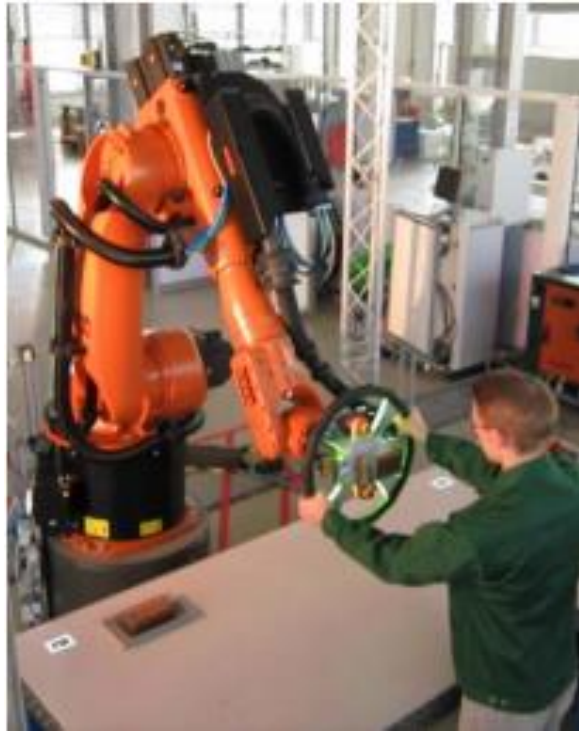
Figure 14 Hand guiding device by Fraunhofer (Fraunhofer 2014a.)
