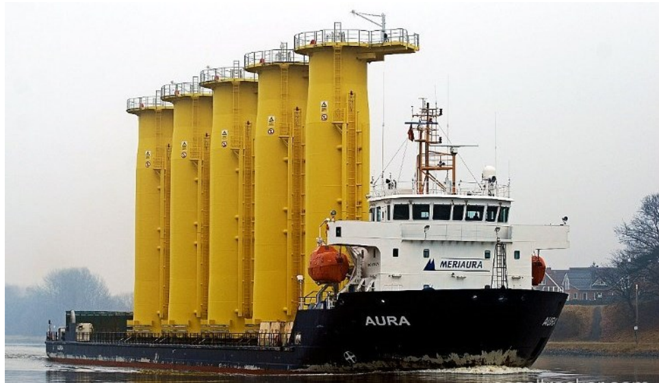
Figure 7 MS Aura transporting very tall wind mill foundations, held in place with Craftmer's securing equipment ( www.meriaura.fi )
