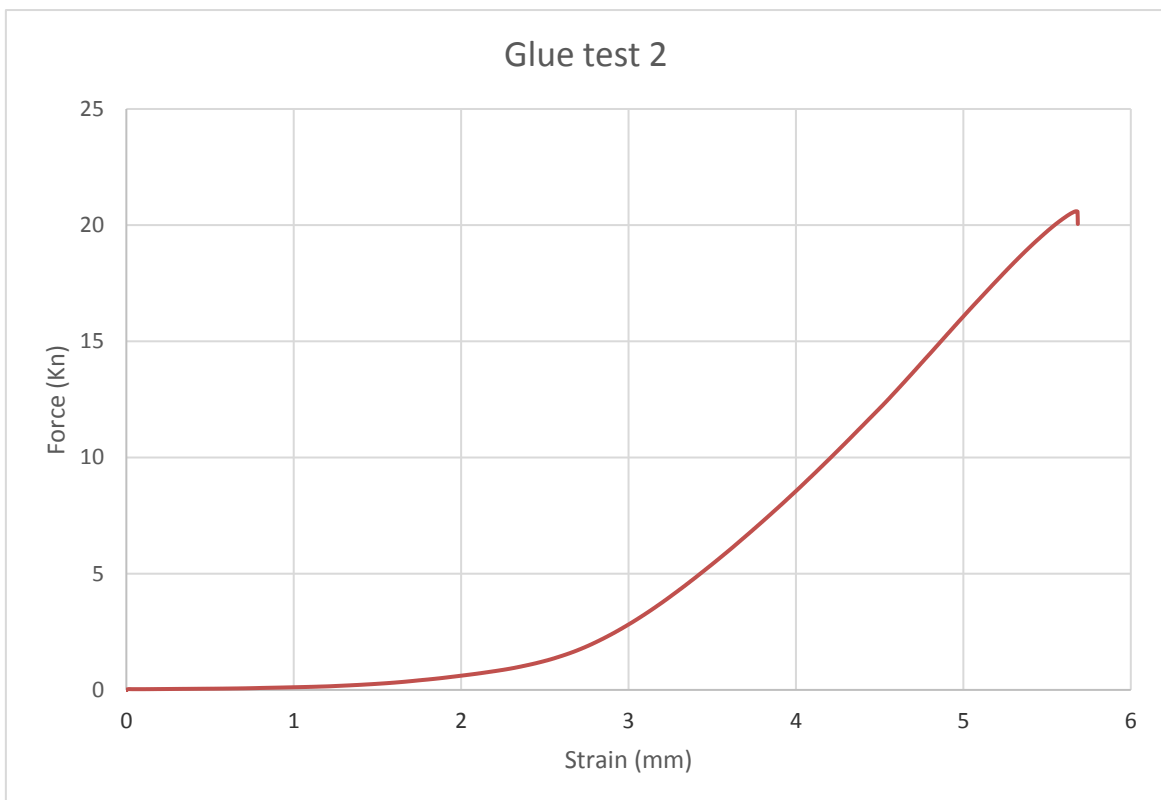
Figure 21. Glue shear test sample 2.
