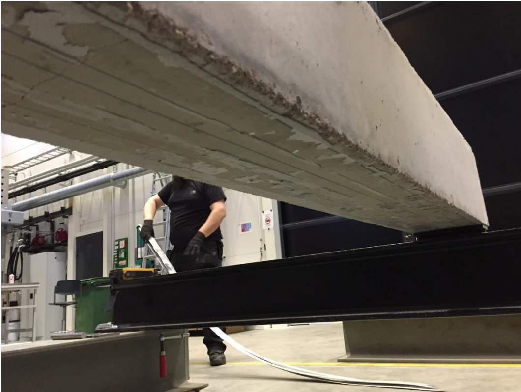
Reinforced beam 2 failure mode
