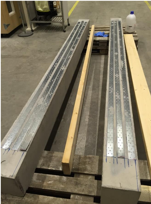
Glued steel plates
