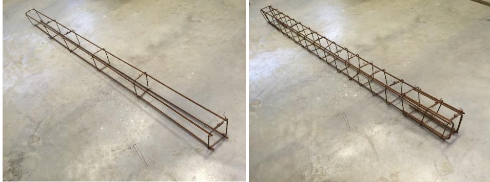
Figure 24. Partially reinforced beam. Figure 25. Fully reinforced beam.
