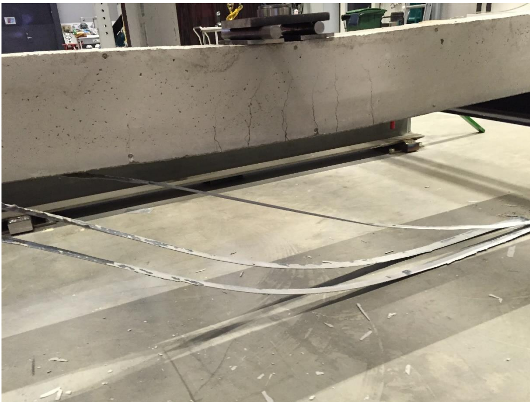
Partially reinforced beam failure mode
