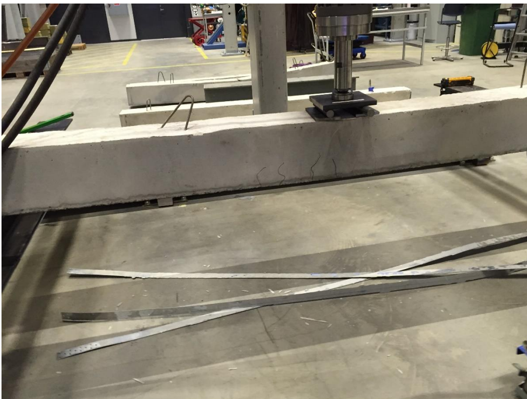
Reinforced beam 2 failure mode
