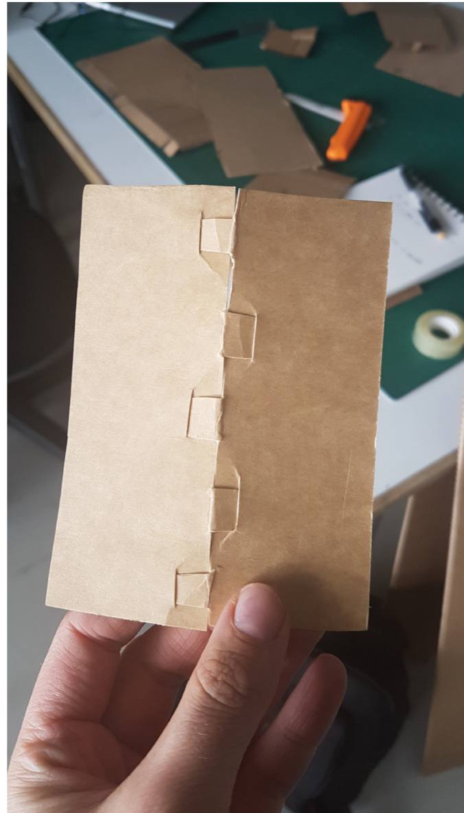
Picture 59 and 60 The left hand picture testing hugging tabs to connect the pieces. The right picture: a different locking mechanism. Backlund 2017.
