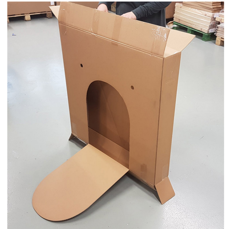
Picture 42. The perforation cut wide open by the factory. Backlund 2017.
