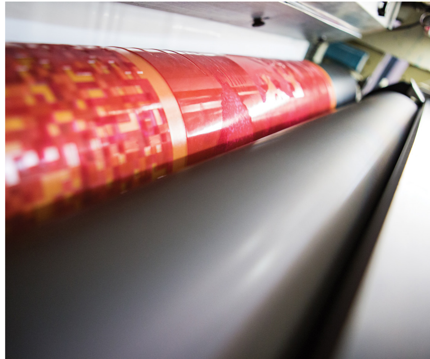
Picture 6. Here the flexo print relief plate is attached to the cylinder. When it's rolled in ink only the protruding parts with the desired design on them will get coloured. anderson-vreeland.ca.
