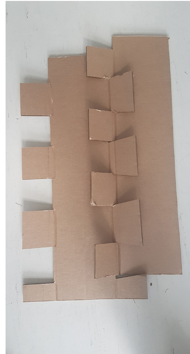
Picture 59 and 60 The left hand picture testing hugging tabs to connect the pieces. The right picture: a different locking mechanism. Backlund 2017.
