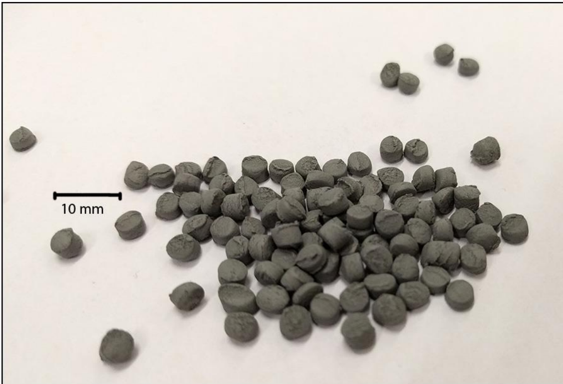
Figure 3. MIM Catamold feedstock granulates, 316L stainless steel (author,2017)
