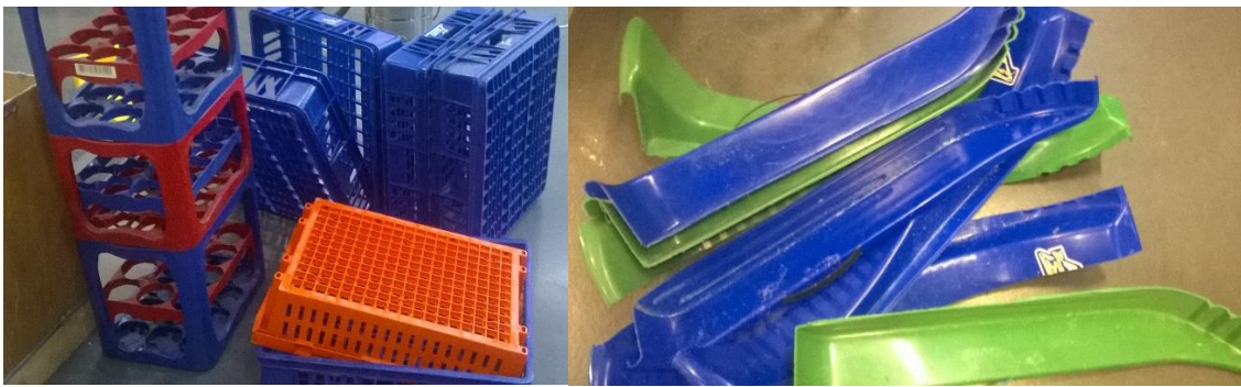
Figure 2: Basket used to make the recycled material, and sledges cut into pieces (The author, 2016)
