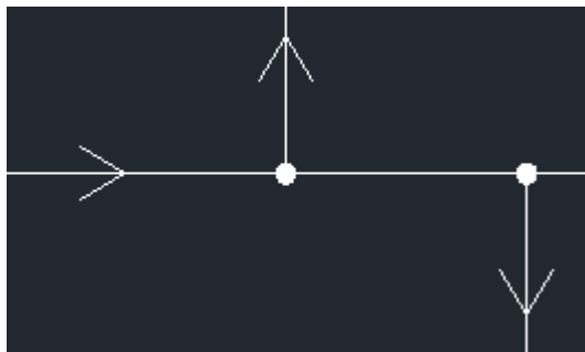
Figure 8. Flow direction arrows after pipe branches
