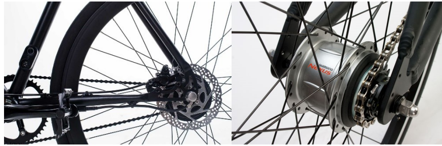
Figure 17. Visual comparison of geared hub motor used in Ampler electric bicycle (Ampler n.d.) versus Shimano geared hub (Montague Bikes 2011)
