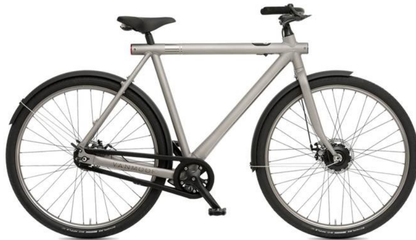
Figure 18. VanMoof electrified S e-bike with built-in frame battery (Treehugger 2016)
