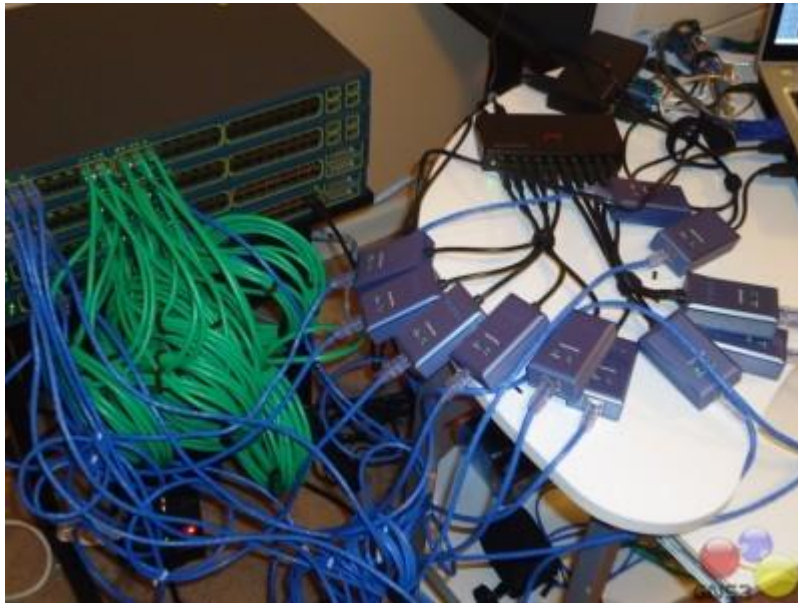
Figure 34. A user preparing to CCIE exams using GNS3, multiple network adapters and physical switches (Ziesemer 2016)
