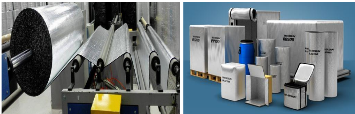
Figure 13. Bubble foil roll and finished commercial products respectively (Courtesy of TP3 Global Ltd.)
