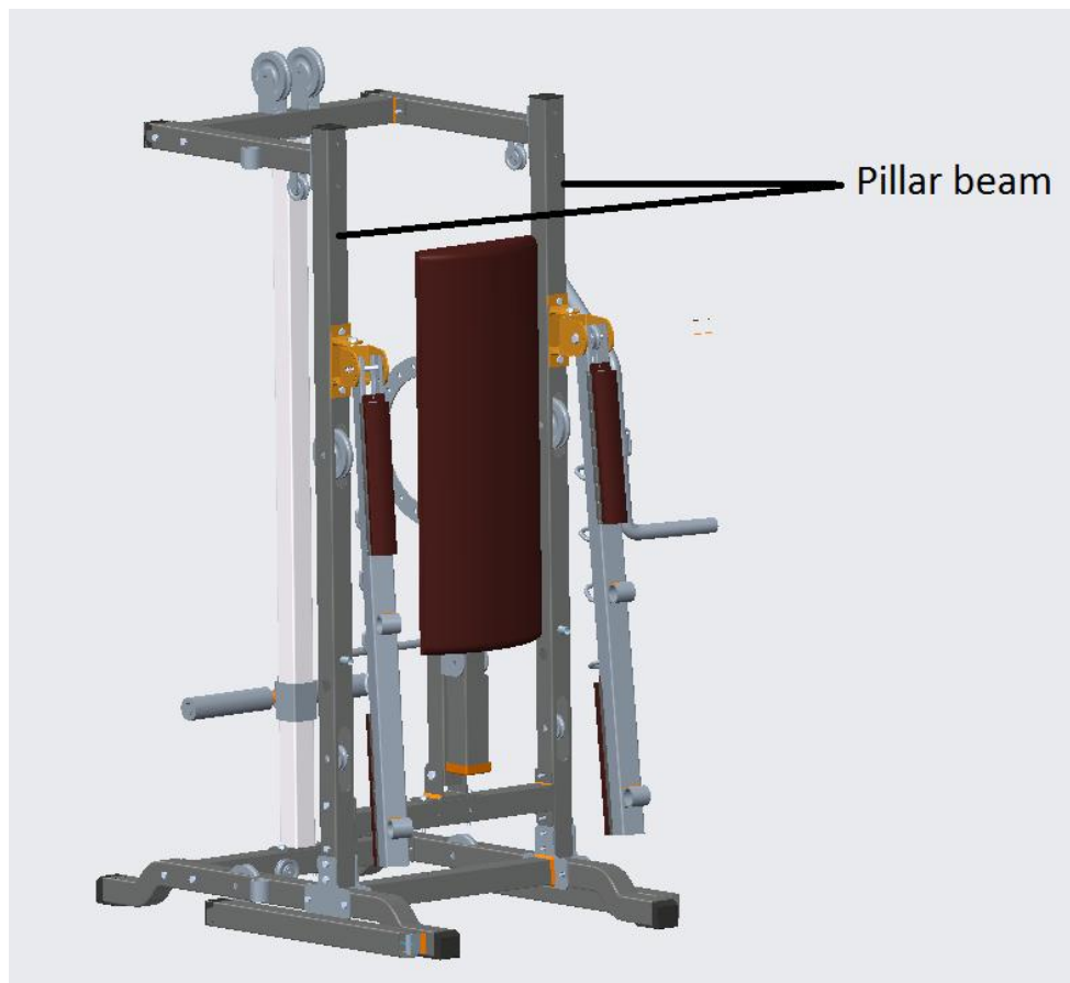
Figure 25. Pillar beam in assembly.
