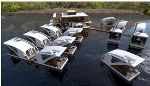
Picture 11. Salt and Water catamarans. These floating catamaran apartments can be docked to a hotel or service station with restaurant or other facilities or it can separately function as an electrical boat. ( http://saltandwater.rs/ ).
