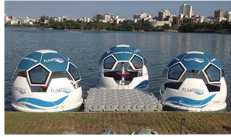
Picture 18. Rental pods. Floating movable “puzzle” quays are functioning as work platforms or as movable platforms for renting “floating capsules” for tourists. ( http://versadock.com/ ).
