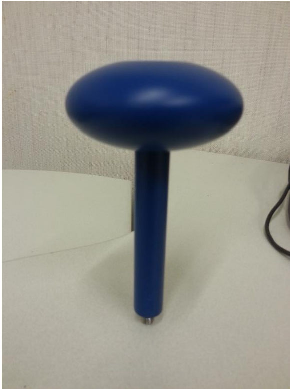
FIGURE 6. A Loop Dipole Antenna. Opposite to a sleeve antenna, radiation polarization will become horizontal if the antenna radiates from this position.
