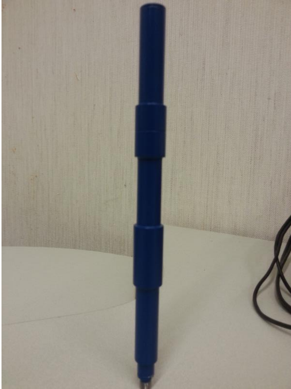
FIGURE 5. A Sleeve Dipole Antenna. Radiation will be vertically polarized if the antenna radiates from this position.
