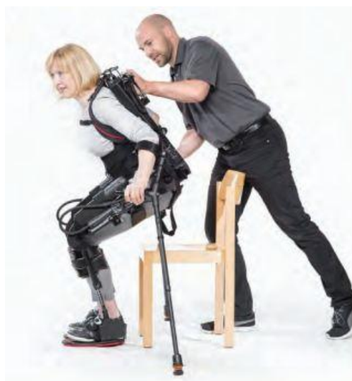
Picture 5. Ekso GT, applying sit-to-stand function (picture is courtesy of EksoBionics).
