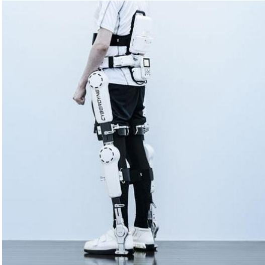
Picture 6. HAL Lower limb exoskeleton for medical use (picture is courtesy of Cyberdyne Inc.).
