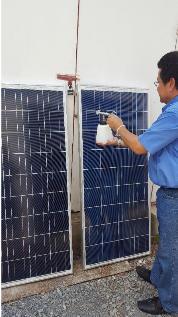
Figure 6. Applying the hydrophilic coating
