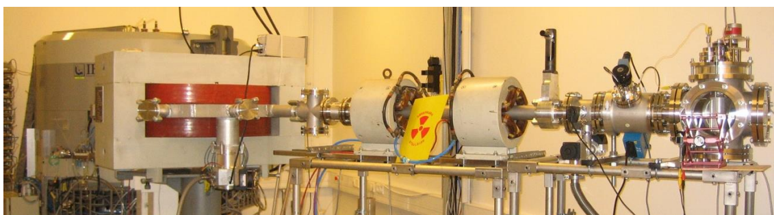
Figure 2. Ion irradiation facility: 5 MeV deuterons were extracted from the cyclotron into an external beamline through a dipole switching magnet and to a target chamber with rolling film holder (right) all under a high vacuum.
