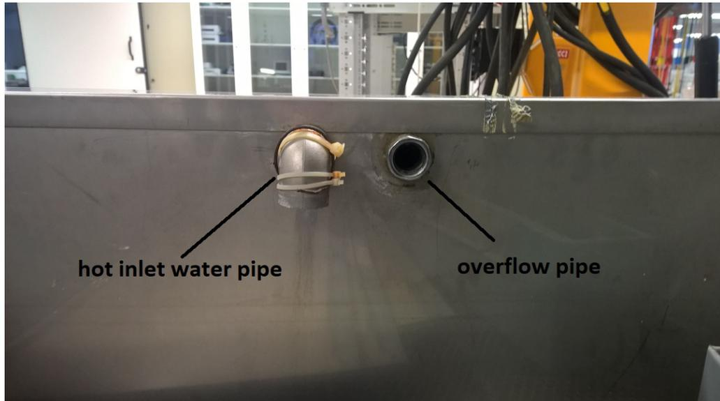
Figure 9. Hot inlet water pipe and overflow pipe (photograph taken by the author)
