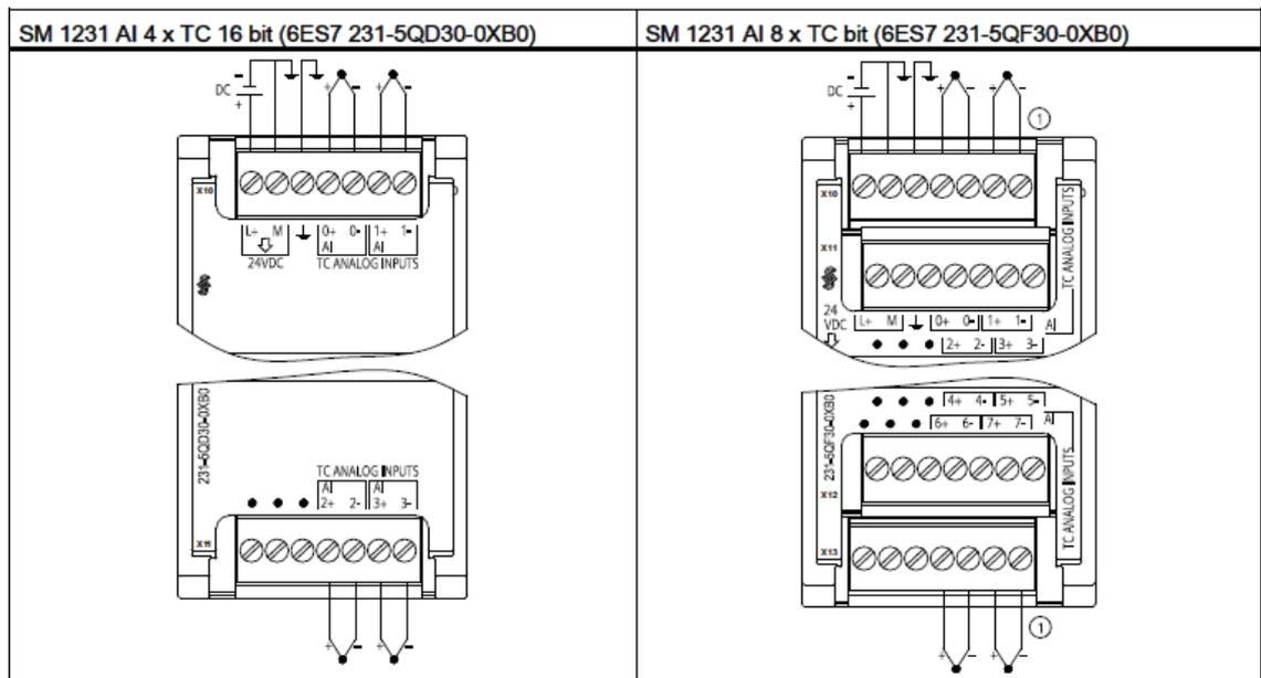
Figure 16. Wiring diagrams for the thermocouple SMs (picture taken from S7-1200 System Manual)
