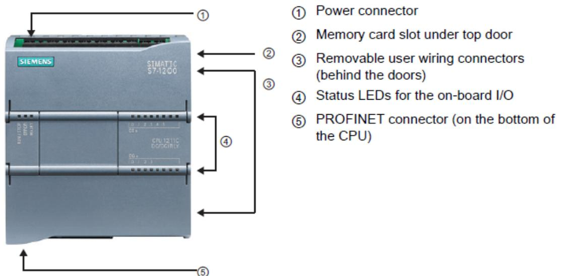
Figure 3. Outline of PLC Siemens 7 1200 (picture taken from page 19 S7-1200 System Manual)
