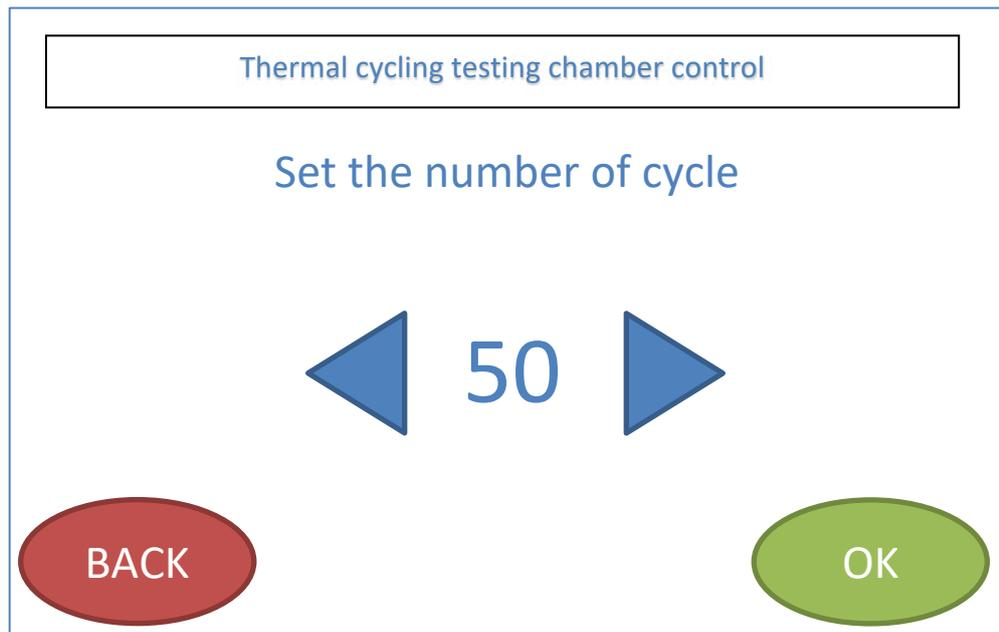
This screen's headline text is "Set the number of cycle". To change the number of cycle, press left or right arrow to minus or add 5 times for each press.
