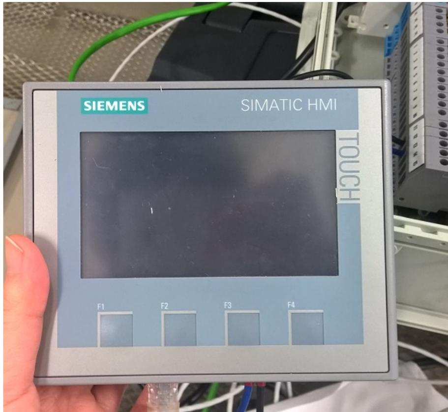
Figure 7. HMI Panel used in this project (photograph taken by the author)
