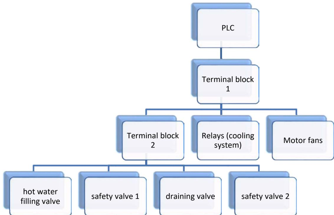
Figure 6. Connection between PLC and instruments
