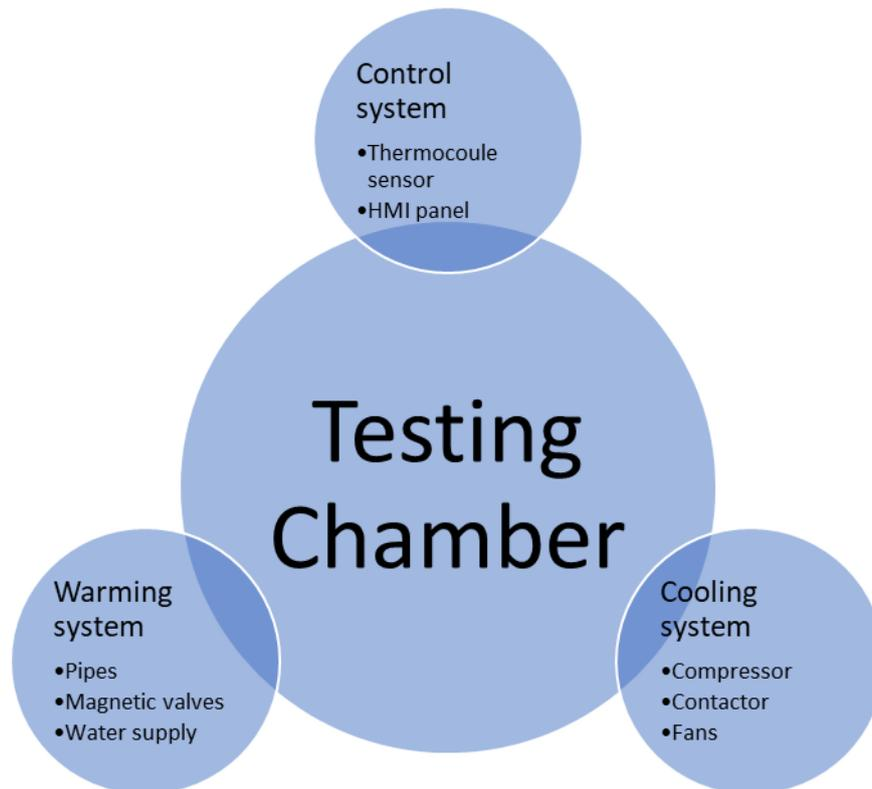
Figure 1. Basic outline of thermal cycling testing chamber (chart created by the author)
