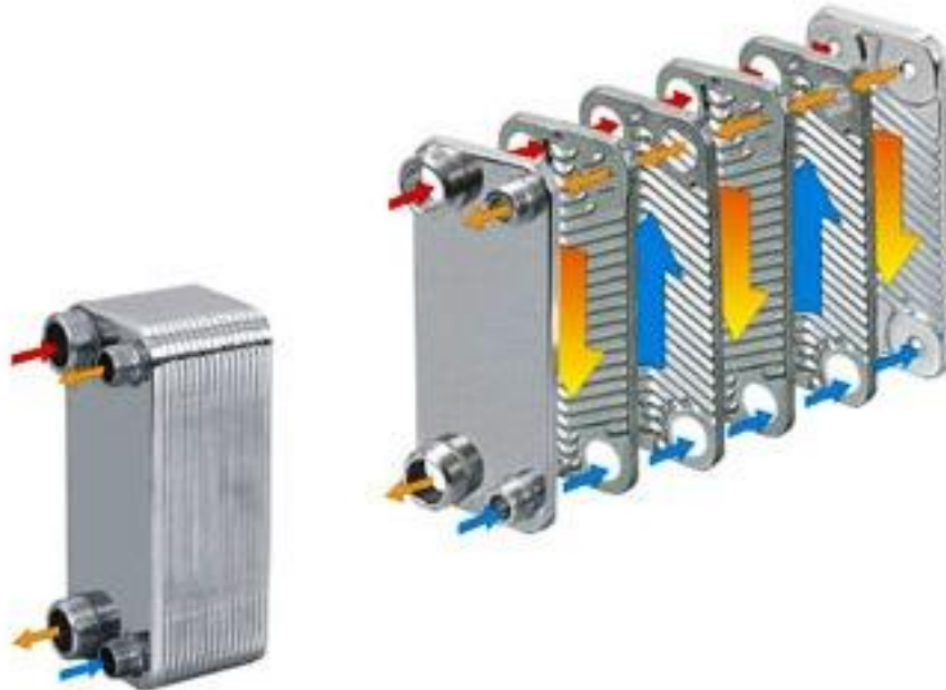
GRAPH 6. Brazed plate heat exchanger (GEA PHE systems 2010)
