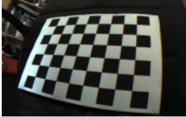
Figure 16: A checkboard used for calibration, the image is taken by Pixy camera that enable clear view of camera distortion.
