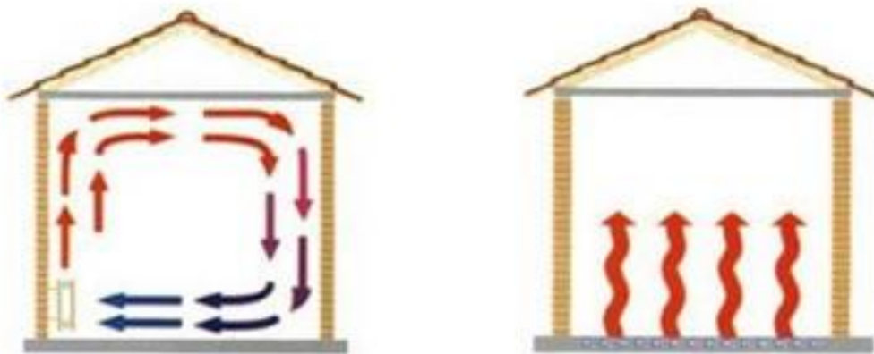
Figure 45. Conventional radiator system vs under floor heating (The Solid Wood Flooring Company 2018)
