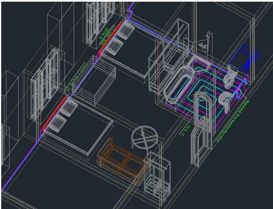
Underfloor heating and radiators in suite
