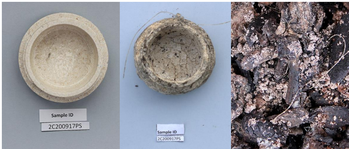
PICTURE 4. Disintegration of the sample No:2C200917PS. On the Left, original sample on 20th of September, before the starting of the test. In the middle, sample 12th of October, after 17 days composting in industrial composting facility. On the right, picture on 21th of November, after 17 days composting in industrial composting facility and 39 days in maturation field. Testing lasted 56 days in total on the composting field. (Petri Sihvonen 2018)
