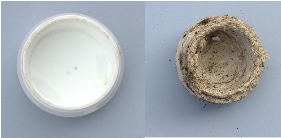
PICTURE 6. Reference sample PlasticM1 on the left. Sample 1G200917PS on the right. Picture on 12th of October, after 17 days composting in industrial composting facility. (Petri Sihvonen 2017)
