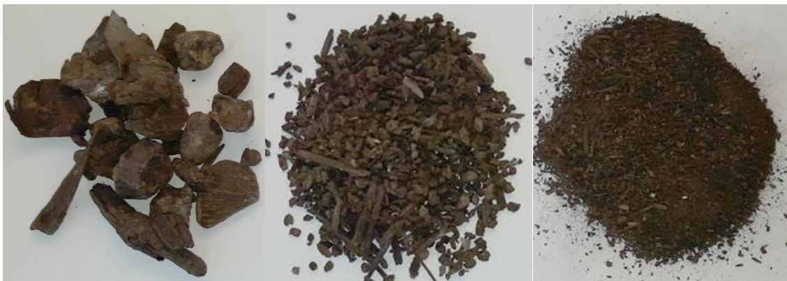
PICTURE 8. Sieving residue; on the left 4 mm sieve, on the middle 2 mm sieve, on the right receiver.
