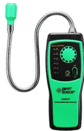
Figure 36 - Gas leak detector (Smartsensor, 2018)
