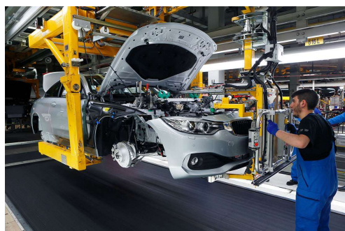
Figure 65 - BMW production. Floor conveyor (BMW AG, 2018)
