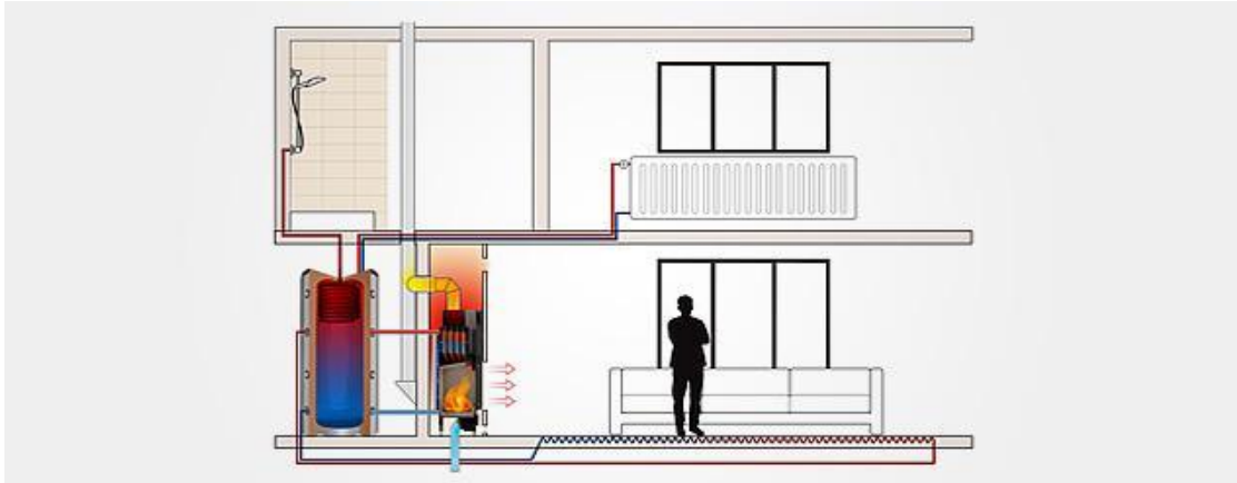
Figure 3. Heating System with Hoxter heating Stove [21.]
