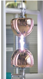
Figure 4: Chopping gaps Figure 5: Spear gaps with surge during the test.
