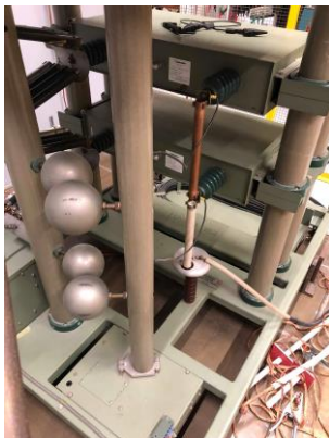
Figure 6: Two chopping gaps (Trigger Electrode)
