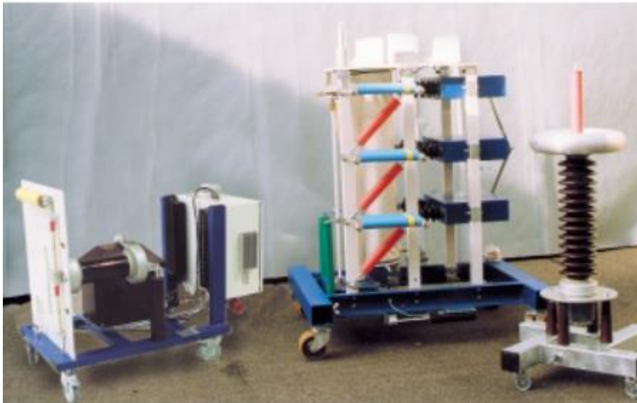
Figure 1: Impulse Voltage Test System SGSA Equipment [3]
